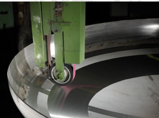
Grinding a stainless steel container
